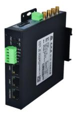
AR7088H Industrial Cellular Router is a kind of terminal device that developed based on 5G/4G/3G/2G, WIFI, VPN technology. It adopts high-powered industrial 32-bits CPU and embedded real time operating system, supports RS232 and RS485, Ethernet and WIFI port that can conveniently and transparently connect one device to a cellular network, allowing to connect to your existing serial, Ethernet and WIFI devices with only basic configuration.
