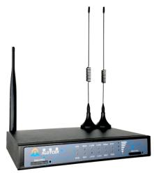
AR7000 Industrial Cellular Router is a kind of terminal device that developed based on 5G/4G/3G/2G, WiFi, VPN technology. It adopts high-powered industrial 32-bits CPU and embedded real time operating system. It supports RS232 (or RS485), Ethernet and WiFi port that can conveniently and transparently connect one device to a cellular network, allowing you to connect to your existing serial, Ethernet and WiFi devices with only basic configuration.
